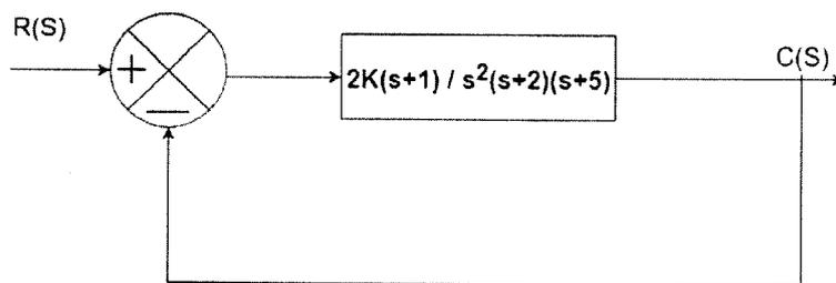
4. For the following multi-loop system, Plot the root locus as  $K_a$  varies from 0 to  $\infty$  so as K.
